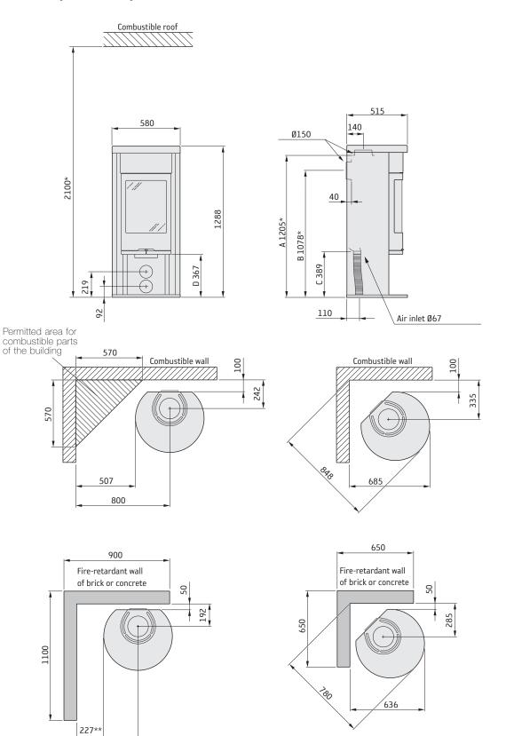
\* If the stove is placed on a hearth plate made of glass for example (accessory), the height from the floor is affected by a distance corresponding to the thickness of the hearth plate, for a free standing glass hearth plate this is 10 mm.
